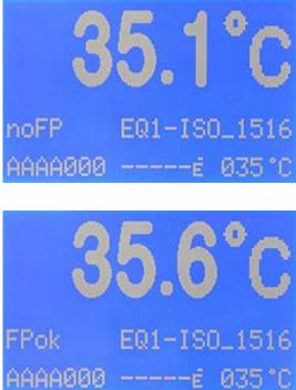
To switch between test conduct according to ASTM D 3934 and ISO 1516 program parameter 30 is set to 0001 (ASTM D 3934, preset as standard setting) or 0002 (ISO 1516).
