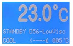
When the temperature goes below the threshold, the signal switches off. On the display "COOL" remains until the <STOP> key is pressed.
