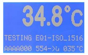
After time expiration a second flash point test is performed. Test is terminated after the second test is finished:
