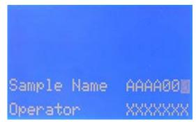
For sample- and user-ID you are given 7 digits which can be used for alphabetical (A to Z) or numerical (0 to 9) signs.
