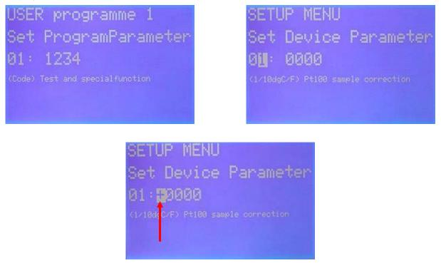
As with the program parameters the number of the parameter will be displayed left and the value on the right. Changes are made with the cursor keys and confirmed with <ENTER>. **The changes will remain permanent even after switching off the device.**
