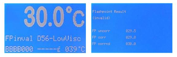
FPnoP02 The flashpoint was detected by a non-standard test. The pre-set cryostat temperature was too high so the auto start temperature could be not achieved or using devices with air conditioning the auto start temperature cannot be achieved because the ambient temperature is too high.
