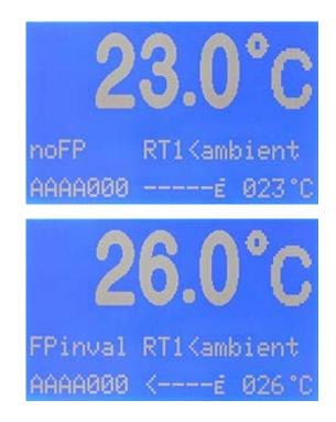
The device cools down to STOP temperature.
