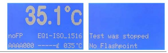
OVERFLO 10°C above the pre-set temperature of the expected flashpoint the program automatically is aborted for safety reasons.
