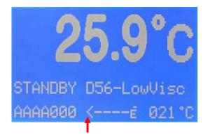
The block will be cooled down to auto start temperature (in the standards 11°C below expected flashpoint). This temperature will be kept for 5 min.
