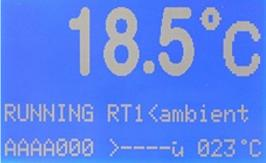
When the filling temperature is reached there will be an acoustic sound for filling the precooled sample with the syringe into the test cup. When the sample was inserted this is confirmed with <ENTER>.
