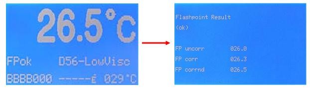
FPok: The detected flashpoint was found in accordance with the relevant standard.
