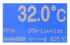
If a flashpoint was detected depending on the compliance with the standards the display shows the following:
