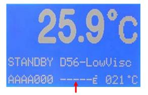
Program has been started. Block is heating. (One bar means approx. 1 min until reaching the test phase.)
