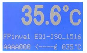
If no flash point is found the test is stopped according to ASTM D 3934 with the following message:
