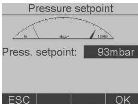
Fig. 6.4: Pressure setpoint with connected Vacuum Pump V-700/710
