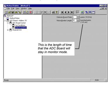
The ADC Board Data Acquisition screen allows you to change the Detector Bunch Rate and Noise Monitor Length. The Detector Bunch Rate sets the frequency of the raw data points stored in the Data File. The Noise Monitor Length specifies how many of the data points will be used to calculate the noise value. The length of time that the ADC Board spends in monitor mode is the product of the frequency of data points and the Noise Monitor Length.
