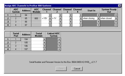
4. The top half of this dialog box is a table for the settings of the analog and synchronization signals. The different rows allow the configuration of analog channels connected to different instruments. ONLY the analog channels connected to detectors in the same instrument should have their settings on the same row. There will be one 800 MIB icon created for each row that has an analog signal setting. Multiple analog signal settings in the same row are different channels in the same ADCB.
