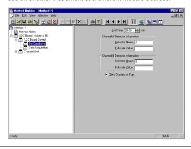
The ADC Board Set Conditions screen allows the user to set the endtime for the ADC Board Data Acquisition. This endtime can also be set from the ADC Board Status and Control Window Endtime... button in System Control. Names for the detectors associated with Channel A and Channel B and their full scale values can be entered for annotation on the printed reports.
