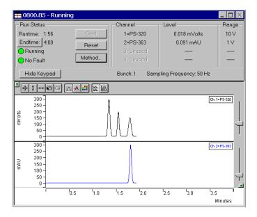
On the left of the Star 800 MIB status window is the Run Status that includes the usual Workstation buttons (Start, Reset, Method Edit and Endtime).
