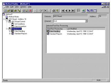
Multichannel detectors can have post-run processing sections for any or all of their channels. For the Method shown above, post-run processing has only be chosen for ADC Board Channel A. The post-run processing for Channel A includes both Data Handling (peak detection and integration) and Standard Reports (numerical results and chromatogram).
